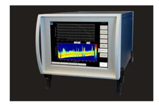
The instruments of the TDEMI M+ receiver series are available for the frequency ranges up to 1 GHz, 3 GHz or 6 GHz starting from 9 kHz each. Additionally these blazing fast measurements can be carried out even starting from 10 Hz optionally (Option MIL/DO-UG).
